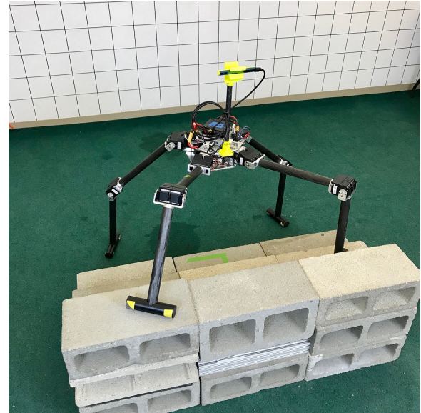
Fig. 1. ALPHRED walking over an unknown terrain by planning based on sampling and optimization.
