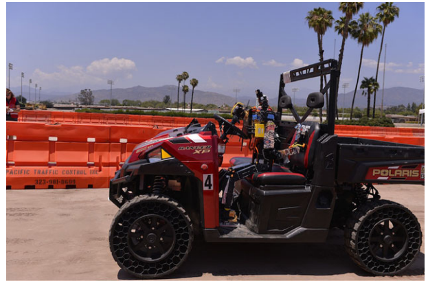
Figure 22. THOR-RD drives the vehicle with its head rotated 180°. Due to the default birdwalk knee configuration, the robot is mounted backward in the car.
