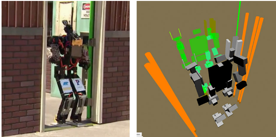
Figure 23. The operator guides THOR-RD through the doorway with the help of LIDAR feedback over the low bandwidth channel.
