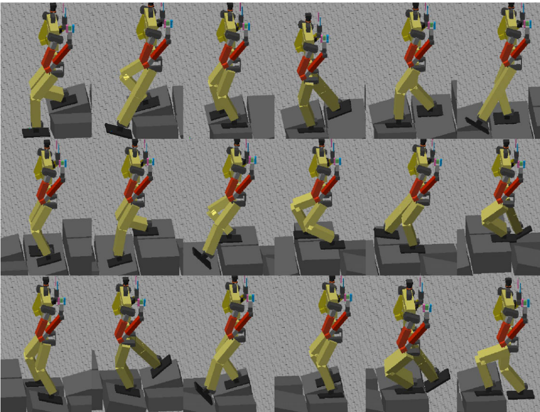
Figure 26. The THOR-RD robot traverses over the DRC Finals uneven terrain in a simulated environment.
