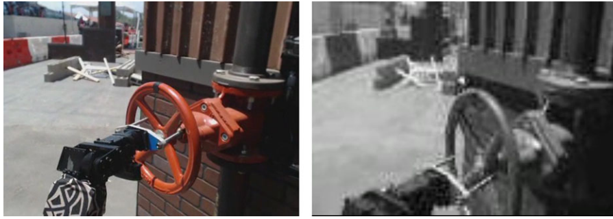
Figure 24. The high and low bandwidth view during the DRC Finals Valve task: The robust passive hand allows for quick alignment, and the low-resolution image feed provides immediate feedback during operation.
