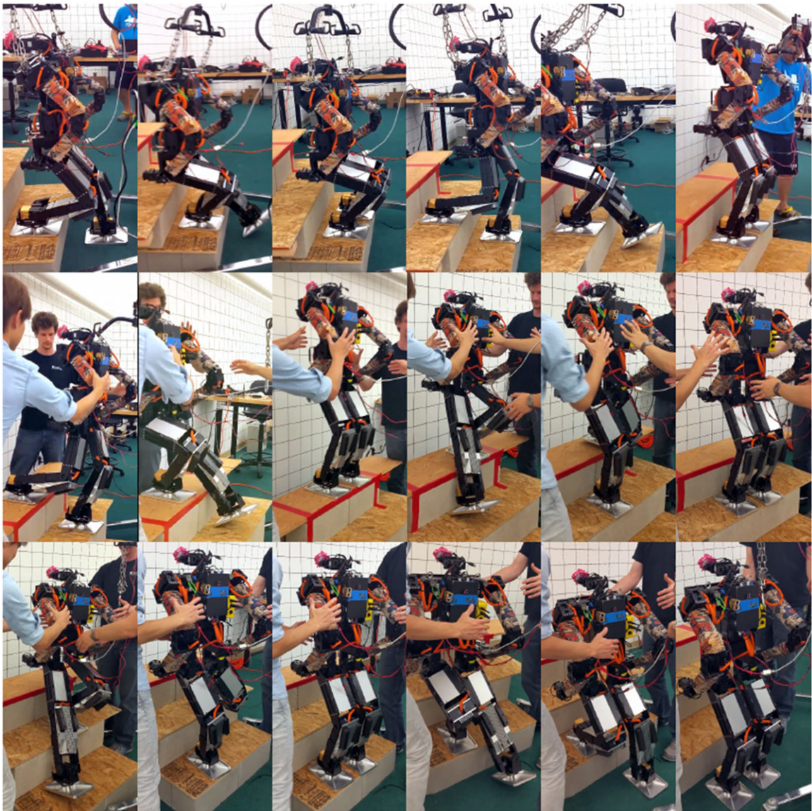
Figure 27. The THOR-RD robot climbing a set of stairs using the toe and heel lift controller.
