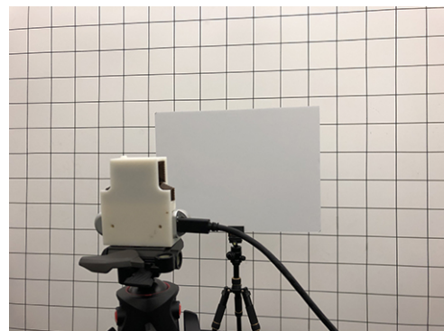
Fig. 6. Actual setup used to gather data at different distances and angles. A distance measurement device with 1.5 mm accuracy was used to measure distances and a video tripod precisely rotated the planar target to the desired angles.
